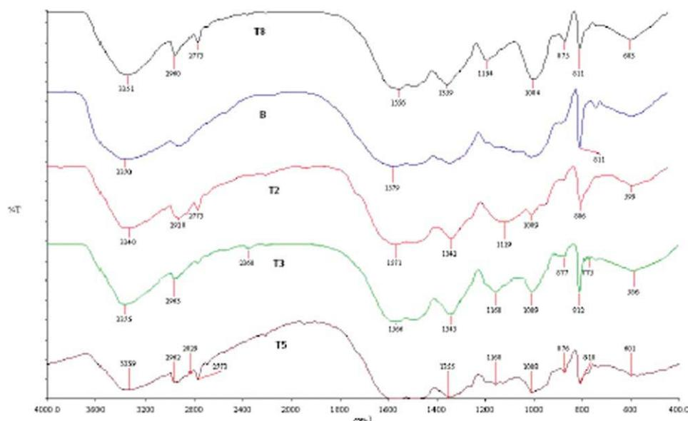
**Figure 4** FTIR spectra of melamine-formaldehyde microcapsules: (K2) 2.5 mole ratio (K3) 3 mole ratio (K5) 5 mole ratio (K8) 8 mole ratio (B) Blank microcapsules. [Color figure can be viewed in the online issue, which is available at [www.interscience.wiley.com](http://www.interscience.wiley.com).]
