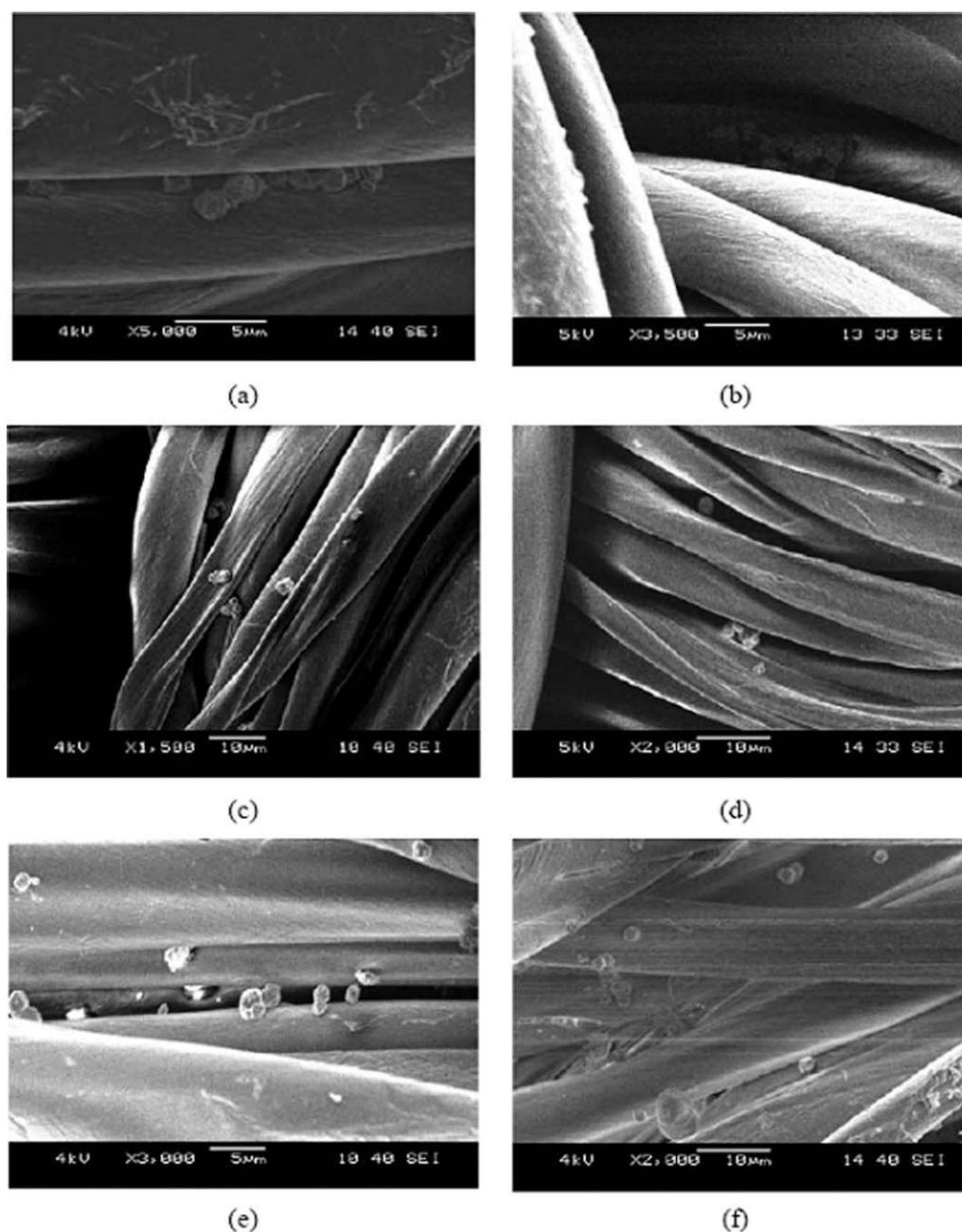
**Figure 9** SEM photographs of cotton fabrics after various washing cycles: (a) 1 washing cycle (b) 5 washing cycles (c) 10 washing cycles (d) 15 washing cycles (e) 20 washing cycles (f) 25 washing cycles.
