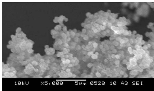
**Figure 2** SEM micrographs of melamine-formaldehyde microcapsules.
