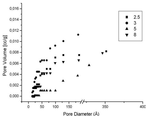
**Figure 7** Pore diameter distribution of melamine-formaldehyde microcapsules.
