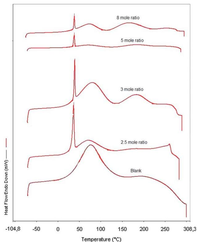
**Figure 6** Thermographs of melamine-formaldehyde microcapsules. [Color figure can be viewed in the online issue, which is available at [www.interscience.wiley.com](http://www.interscience.wiley.com).]
