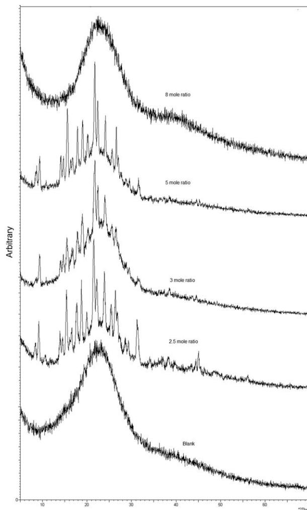
**Figure 5** XRD patterns of melamine-formaldehyde microcapsules.
