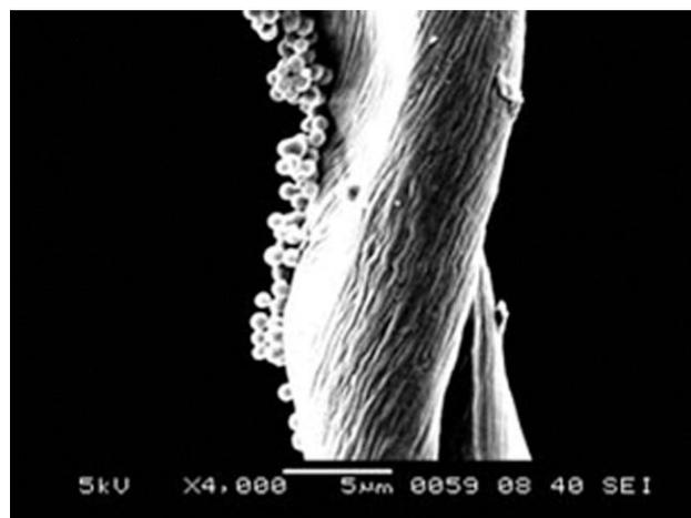
**Figure 8** Attached melamine-formaldehyde microcapsules onto cotton fibers.
