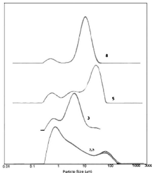
**Figure 3** Particle size distribution of melamine-formaldehyde microcapsules.
